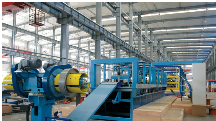
Fully automatic robotic lamination machine
